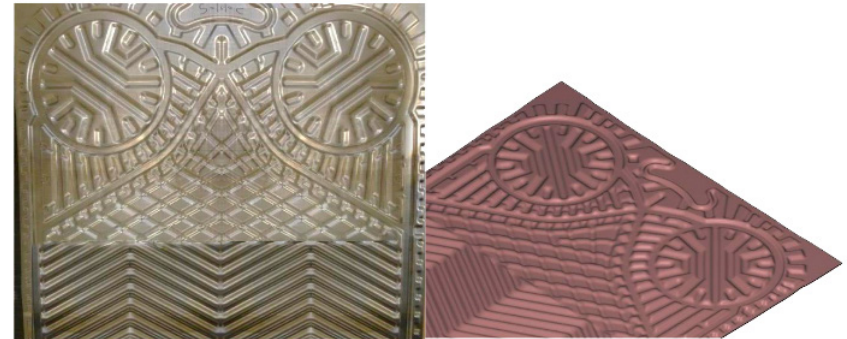
Figure 3. Formed GPHE plate and final configuration from Finite Element Analysis.
